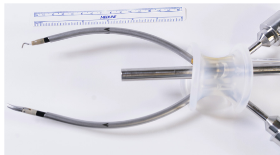
Fig. 1 – The robotic single-site port viewed from above. Dissection was primarily performed with a hook electrocautery and a Maryland dissector. Intelligent programming permits the hook electrocautery to be controlled by the surgeon's right hand, despite it being inserted through the left side of the port and being controlled by the left-sided robotic arm. (Color version of figure is available online.)
